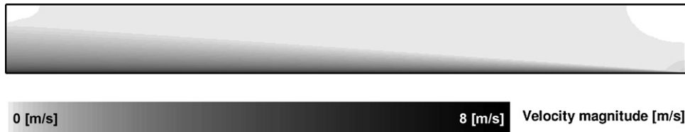
Fig. 2. Contour plot of absolute velocity above a moving wall (2D-simulation). Domain size: 5 m × 0.5 m. Speed of moving boundary: 8.33 m/s. Direction of movement: from right to left. At the white areas (top left and top right) the absolute velocity is less than 1% of the wall velocity.
